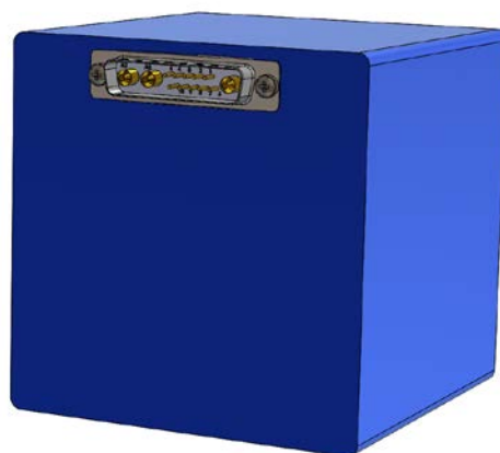
Figure 4 1U Experiment Cube with protruding male DB13W3P connector
