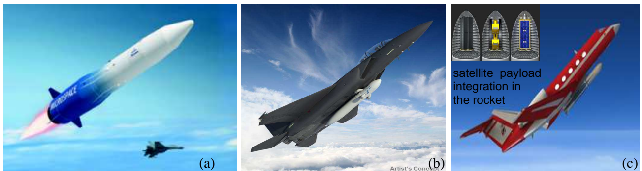
Fig 5:(a)Microspace-2 project (Russia)-40kg payload to 1000km orbit,(b)ALASA project (USA)-45kg payload, (c) GOLauncher 2(USA)-45kg payload using a modified LearJet35,possible orbits ~1000km, inclination 0-98.7 deg
